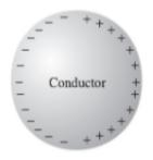
If you hold a charge +q near an uncharged conductor, the two will attract one another. The reason for this is that q will pull minus charges over to the near side and repel plus charges to the far side. The charges move around in such a way as to kill off the electric field inside the conductor. Since the negative induced charge is closer to q, there is a net force of attraction.
