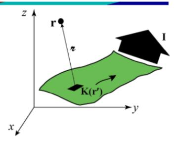
The magnetic field produced by a volume current
