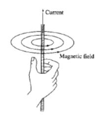
When defining of the electric field, the electric field strength can be derived from the following relation:  $\mathbf{E} = \mathbf{F}/q$ . Since an isolated pole is not available, the definition of the magnetic field is not as simple.
